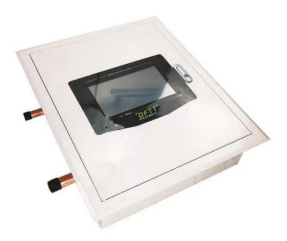
DFTT® Medical Gas Valve Box is used for Gas monitoring, often used in hospitals, where Medical staff control the Gas flow in each ward. Medical Gas valve box is a Medical Gas area valve box, including a box, a door, a lock and at least one valve set. Each valve set includes a sequentially connected inlet pipe, valve, intermediate pipe, barometer and outlet pipe. The front end of the box body is provided with a maintenance port, and the box door can be opened and closed with the maintenance port.
